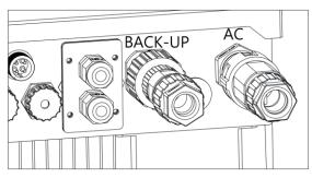
Loosen the cap on the terminal, pull the threaded sleeve out of the socket.
