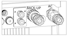
Remove the AC connector: Press the bayonet out of the slot with a small screwdriver or the unlock tool and pull it out, or unscrew the threaded sleeve, then pull it out.
