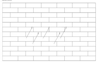
Insert the expansion tubes into the holes and tighten them. Install the bracket with the expansion screws.
