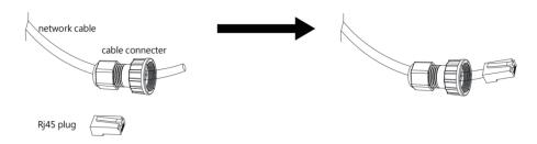
Step 4: Insert the cable connector into COM port at the bottom of inverter and screw it tightly. Then insert other side of the network cable into PC or other device.
